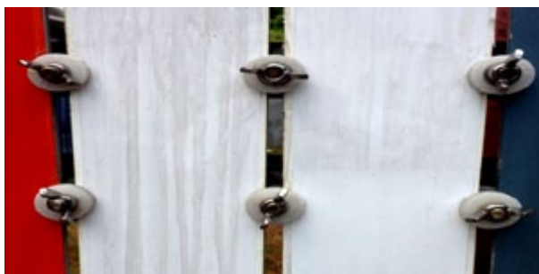
普通涂料与自清洁涂料降雨后“雨痕”对比 The rain print comparison between the surface using normal coatings and that of using self clean paint
